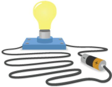
**Lengthening the wires** in a simple circuit will reduce the electrical energy, as it has further to travel. The extra distance will make the bulb **dimmer**.
